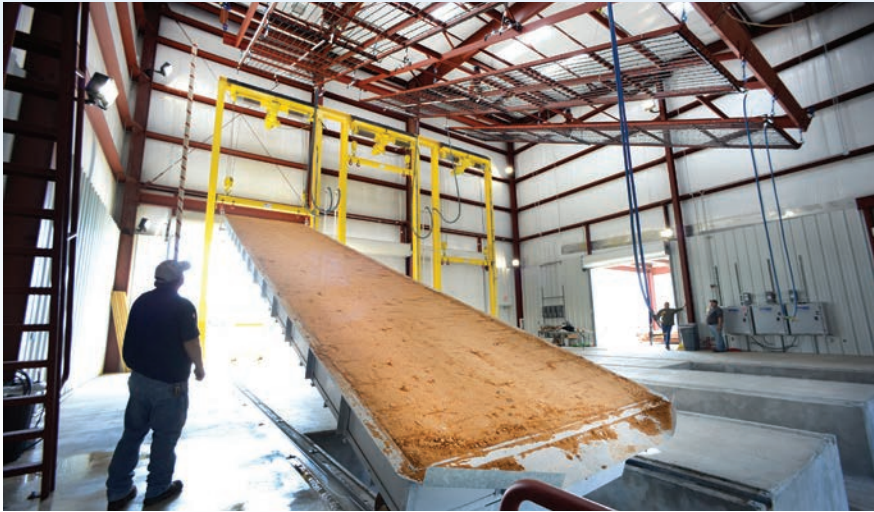
TTI researchers used soil-filled test beds, shown here, to measure soil loss and evaluate the effectiveness of erosion control products.
