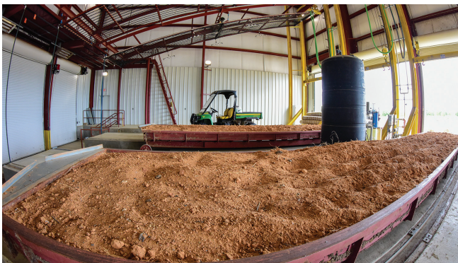
The SEC Lab houses five indoor rain simulators, a physical property test lab, a 1,000-foot vegetated natural soil embankment, a variable slope channel flume, a sediment control device evaluation facility and pollinator test plots.
