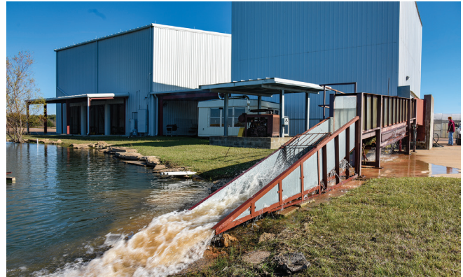
The 30-foot outdoor variable slope channel flume is used for evaluating the performance capabilities of flexible channel liner materials at a range of shear stress flows.
